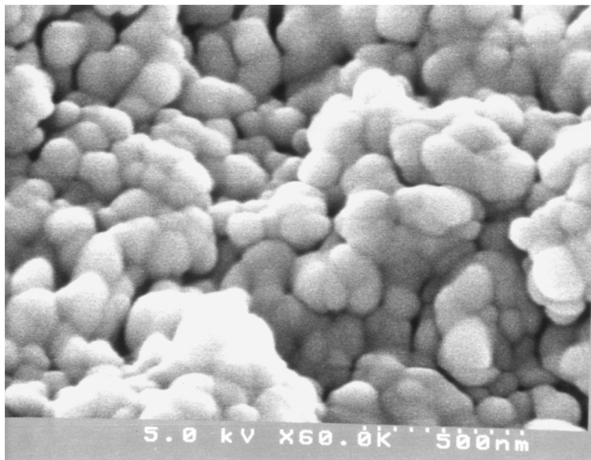
Figure 5 SEM micrograph of \text{TiO}_2 coating on glass bead after eight coating/heat treatment cycles.
